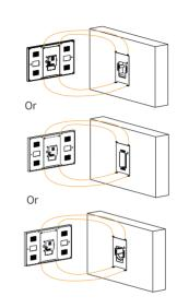
Tilt the device 15° and align the grooves on the back cover with the hooks on the bracket.
