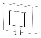
Use Allen wrench fix two M2x5 hex socket screws into the bottom of the device. And the installation is done.
