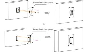
Fix the wall-mounting bracket on the 86 embedded box with two M4x20 crosshead screws, please ensure the bracket against to wall.
